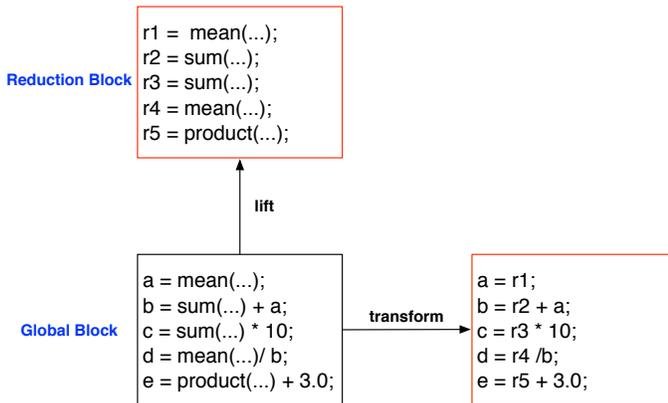
Fig. 10: Reduction lifting makes it easier to group reductions when generating target code. Each reduction is replaced with a new variable in the expression and is lifted into a special code block for reductions.
