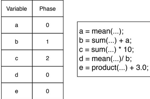
Fig. 9: Reduction variables are assigned into phase groups for execution. A phase group for a variable is incremented depending on whether other reduction variables reside in the same expression. This process greatly reduces the amount of overhead of performing a reduction versus individual execution.
