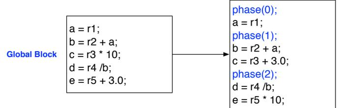
Fig. 11: Phase execution calls are inserted before the execution of the assignment that uses the reduction.
